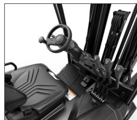
Manual lever hydraulic control.
