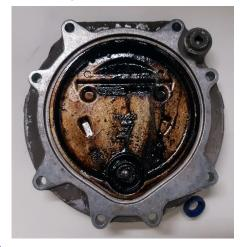
LPG fuel containing contamination not present historically is being placed on the UK market. The fuel standard BS 4250 does not provide adequate controls for this contamination.
