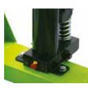
MAX PRESSURE VALVE When maximum load capacity is exceeded, the oil pressure exceeds its maximum limit and the valve automatically stops the forks from lifting. In this way, possible structural damage is avoided.
