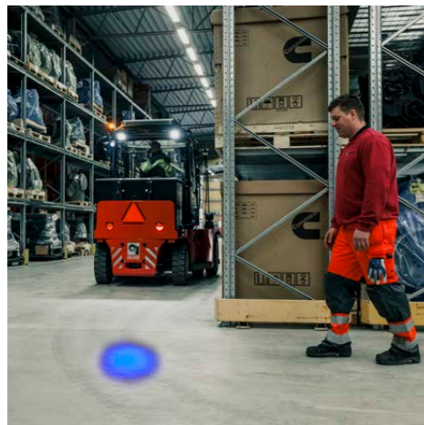
Blue safety light The blue safety light alerts people that the truck is approaching, reducing the risk of accidents.
