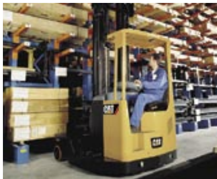
(Left) Compact and heavy duty chassis options. (Right) The multi-way reach trucks are designed for handling long loads.
