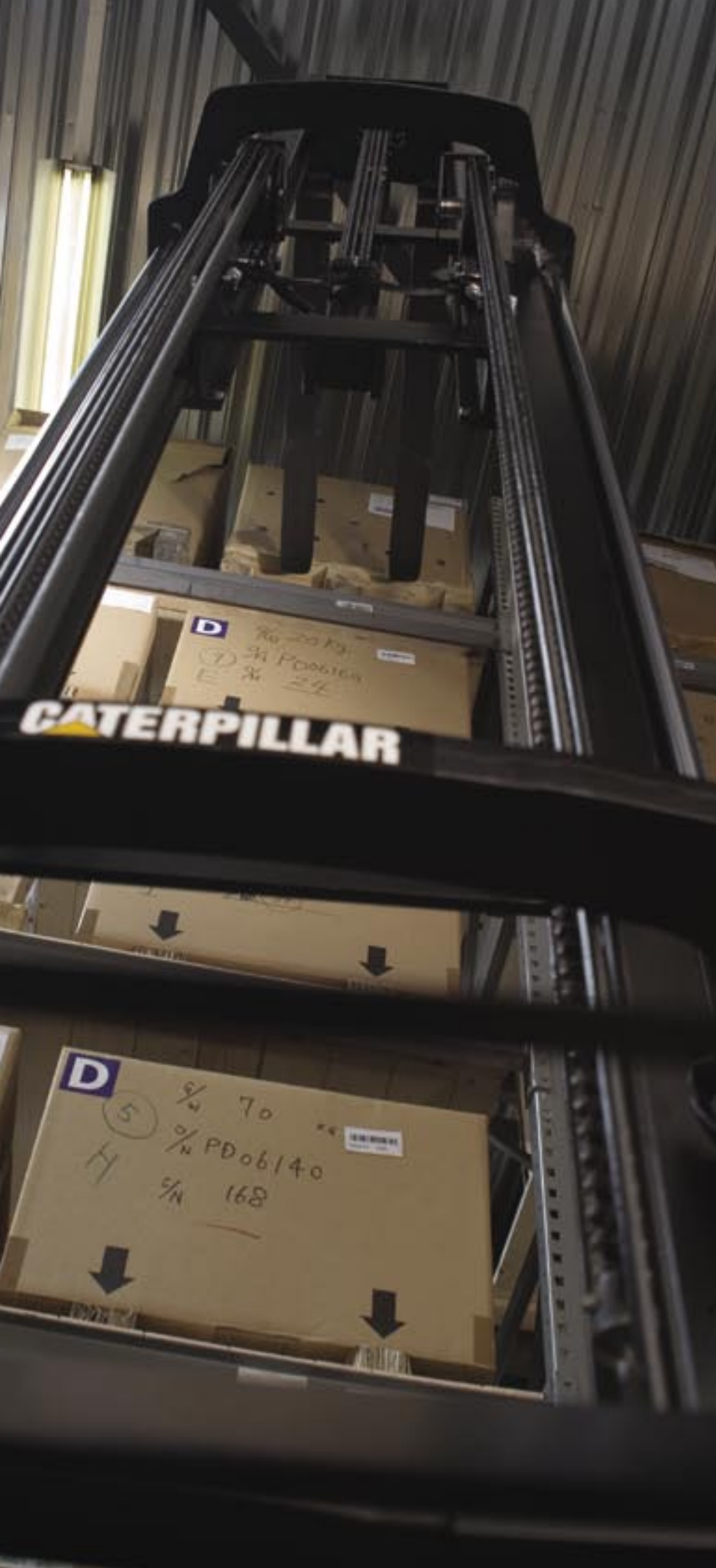
Dramatically improved operator's view ( left & above ) with carefully placed cables and hoses ( above ) and the hydraulic cylinders incorporated within the mast profiles ( far left ).
