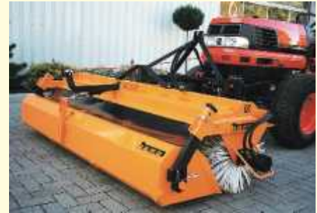
bema 20 Tractor mounting with 3 point front mounting
