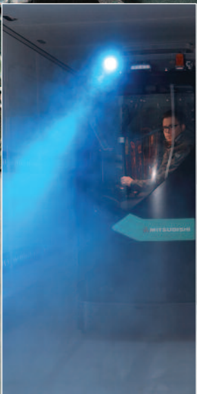
Pedestrian warning system
