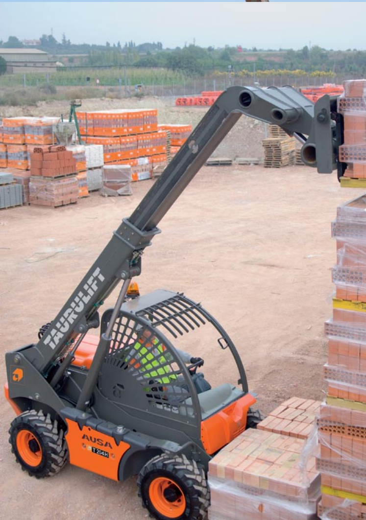
Chasis support for fork lifting (Optional T133/144 H)
