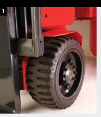
1 Cushion rubber tyres ensure that Flexi performs as efficiently outdoors as it does in the warehouse.
