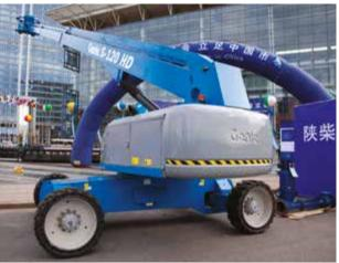
The horizontal outreach of the Genie Super Boom line is among the industry's best at 22.86 to 24.38 m (75 to 80 ft), depending on the model.
