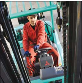
Clear view through mast
